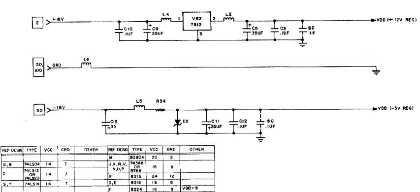
Figure 3-18. CPU Voltage Regulator Schematic
