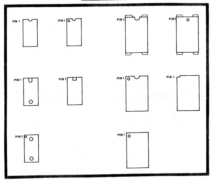
INTEGRATED CIRCUITS (IC's) CAN COME WITH ANY ONE OF, OR A COMBINATION OF, SEVERAL DIFFERENT MARKINGS. THESE MARKINGS ARE VERY IMPORTANT IN DETERMINING THE CORRECT ORIENTATION FOR INSTALLATION. REFER TO THE ABOVE DRAWING TO DETERMINE THE POSITION OF PIN 1 OF THE IC AND USE THIS INFORMATION TO ORIENT IT AS DESCRIBED IN THE ASSEMBLY MANUAL.
