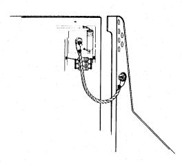
NOTE: At any point where a connection is made to the chassis, first rub the area around the connection point with sandpaper or some other abrasive to remove the anodizing.
