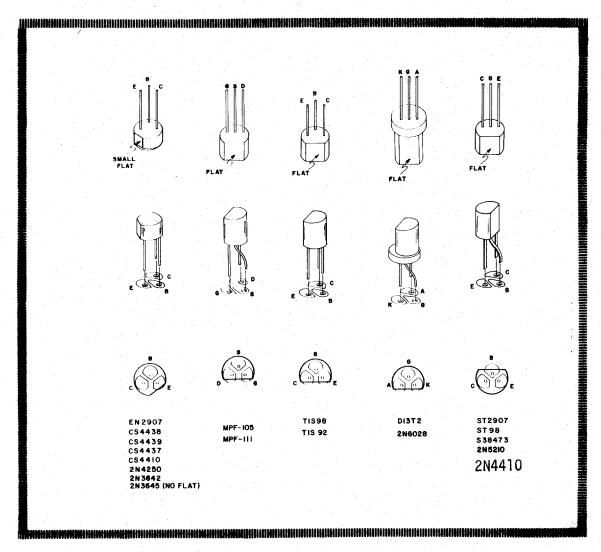
IN THE ILLUSTRATION ABOVE THE OUTLINE OF EACH TYPE OF TRANSISTOR IS SHOWN OVER THE PADS ON THE CIRCUIT BOARD WITH THE CORRECT DESIGNATION FOR EACH OF THE THREE LEADS. USE THIS INFORMATION TOGETHER WITH THE INFORMATION IN THE ASSEMBLY MANUAL FOR THE CORRECT ORIENTATION OF THE TRANSISTORS AS YOU INSTALL THEM.
