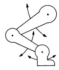
This is a simplified sketch, but it shows that only three moves are required to make the leg functional. Each section of the leg can be treated as "Lever B" in the double windlass mechanism described here. Each section can be powered and controlled individually, drawing power from the single main motor.
